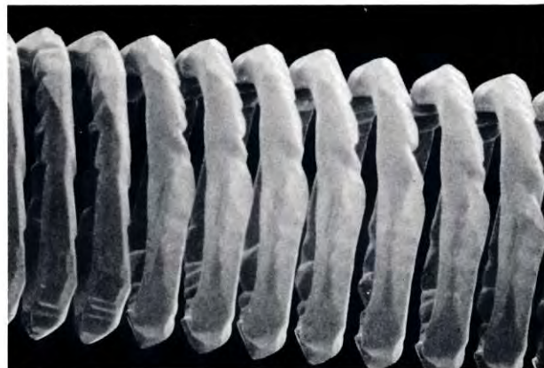
An example of filament notching.
