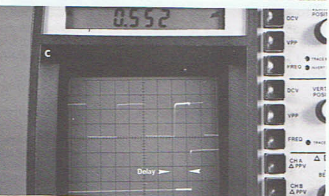
Fig. 56 — To measure the delay between two signals: (A) Adjust the Delta Begin control until the bar is on the top waveform transition, (B) Adjust the Delta End control until the bar is on the bottom waveform transition, (C) Read the delay on the digital display.
