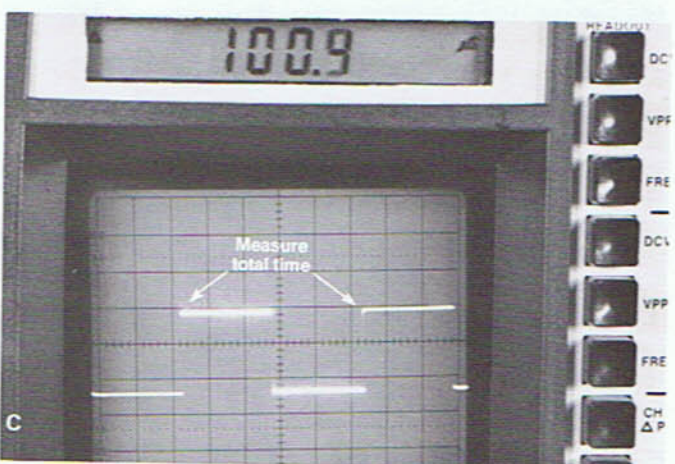
Fig. 55 — Duty cycle is measured by comparing the on-time to the total time of a waveform. Note that only one Delta position needs to be changed to expand the Delta Bar.
